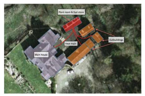
An alternative solution may be to install an Energy Cabin (a pre-configured plant room within a container which can be clad in sympathetic material). This can be craned into position on a prepared concrete slab, subject to the constraint of crane vehicle access.
