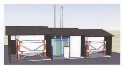
The plant room will house 2 x KGT2626 fuel silos in each outer section, with the boilers, accumulator tank and expansion vessel in the middle section.
