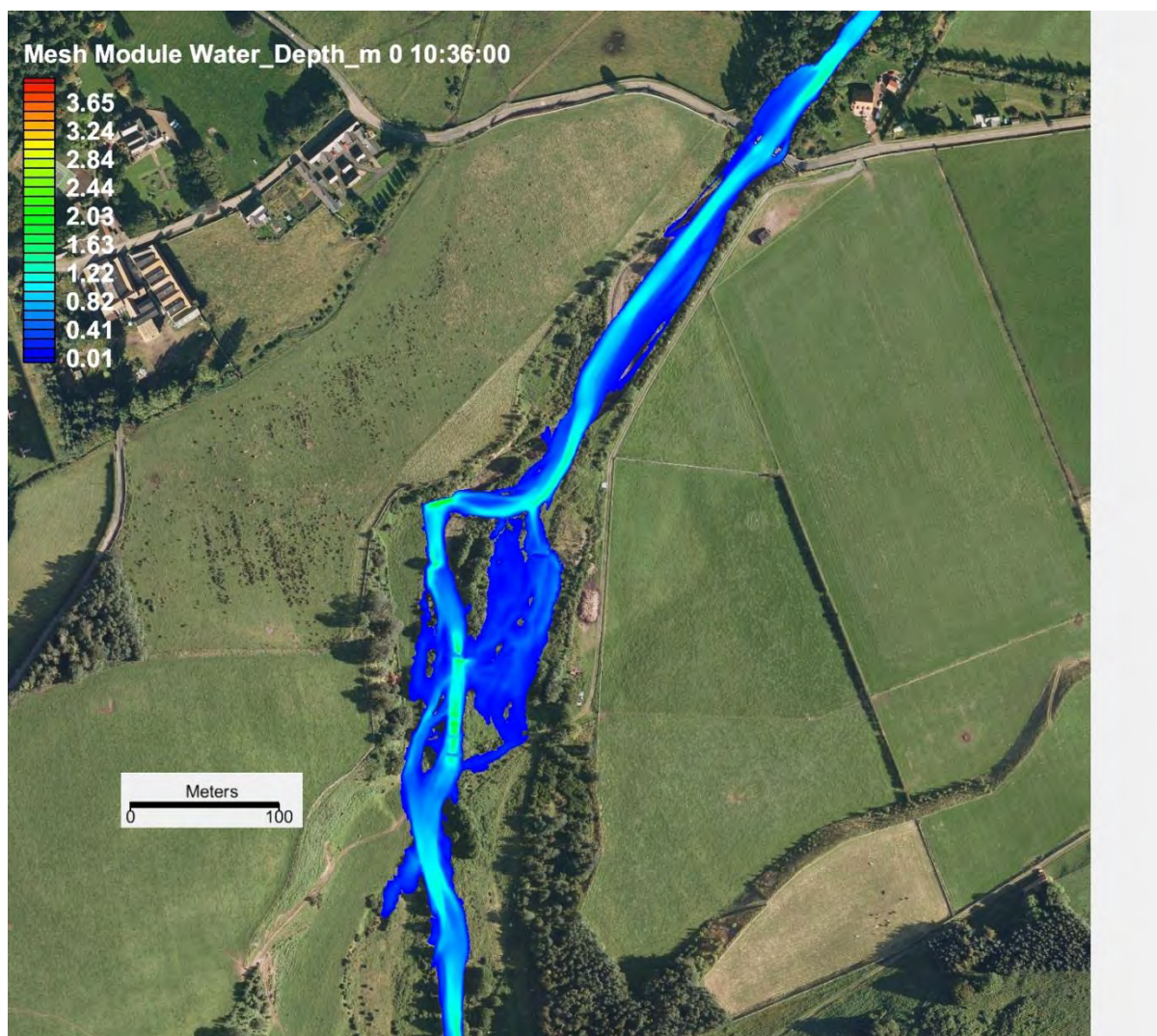
Figure 2.14. Water depth for existing conditions computed at a discharge of 26cms (~ Q_{2yr} peak) during the Q_{200} year hydrograph
