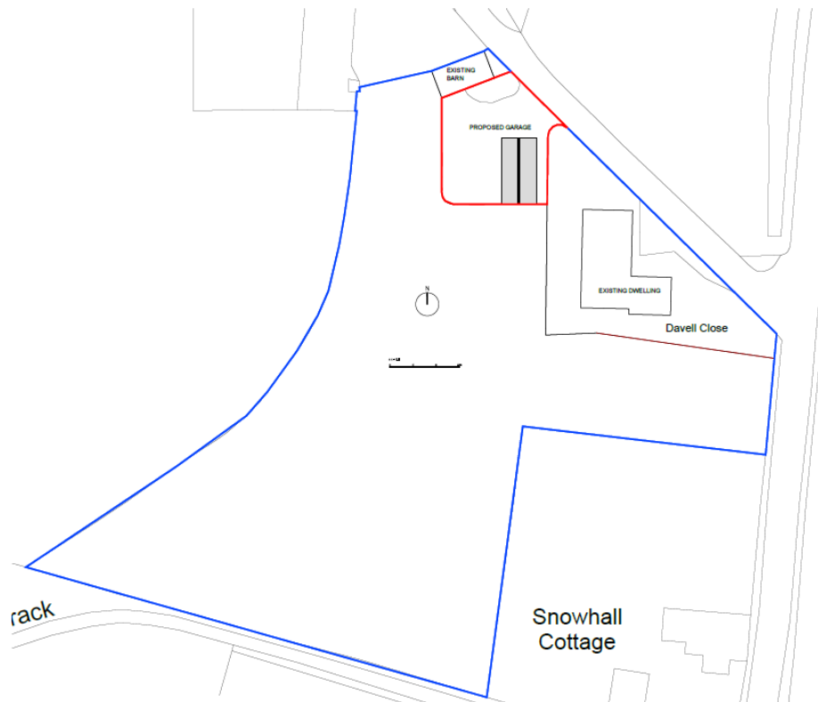
Proposed site plan showing existing property and garden (outlined in black) and application site (outlined in red)
