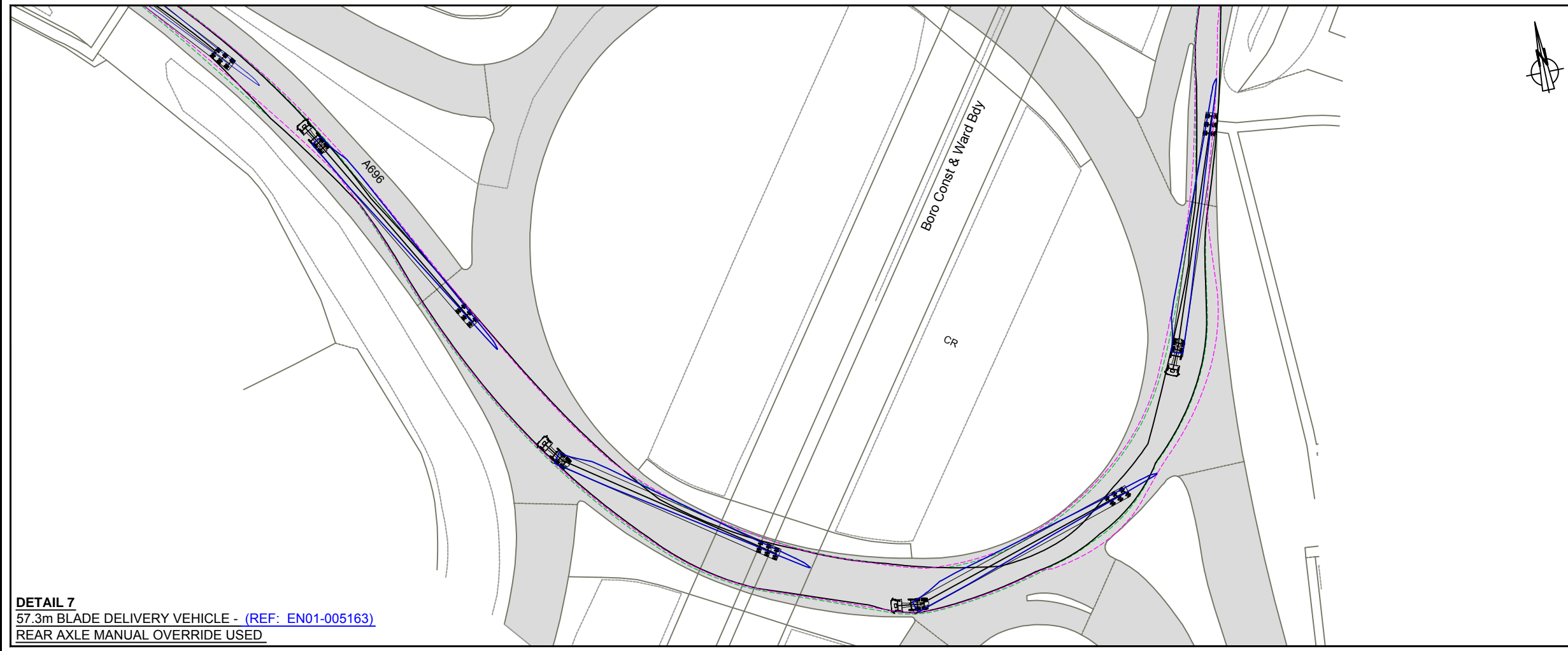
DETAIL 6 57.3m BLADE DELIVERY VEHICLE - (REF: EN01-005163) REAR AXLE MANUAL OVERRIDE USED
