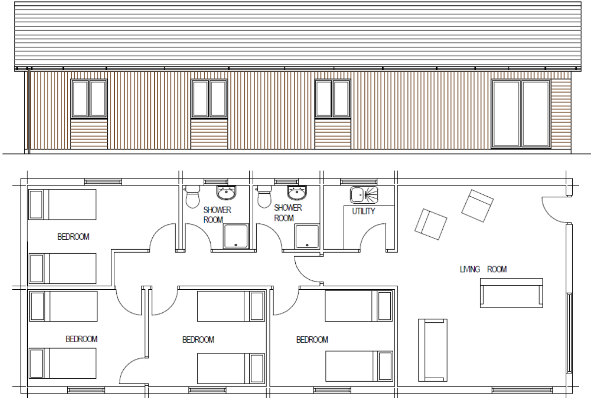
Fig. 3: Proposed bunkhouse west elevation and floor plan
