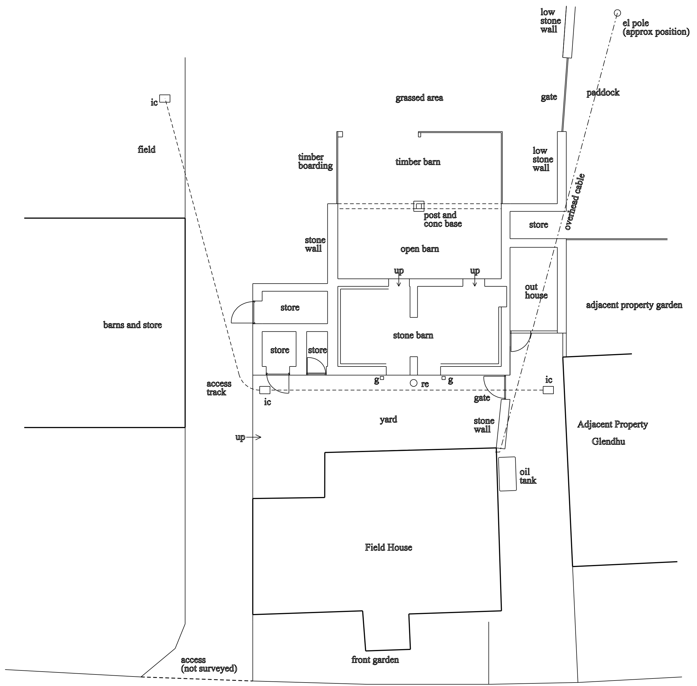
existing barn floor plan 1:100 scale
