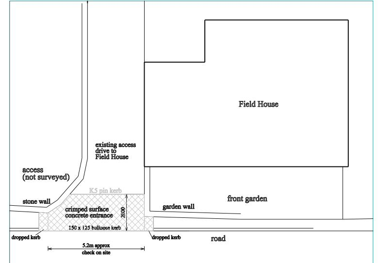
proposed Type A access plan 1:100 scale
