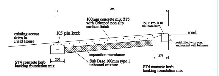
Type A construction section 1:20 scale
