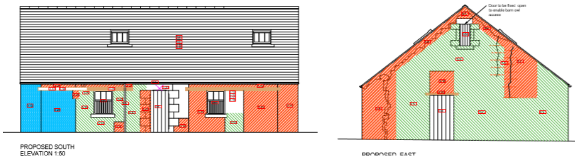
Figure 3: Proposed areas of intervention to the southern (left) and eastern (right) elevations
