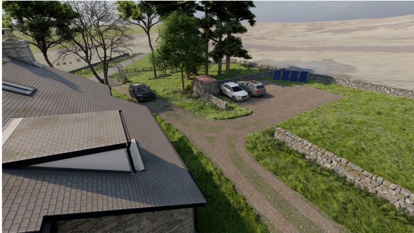
Fig.43 3D visual - aerial view of turning head and discrete parking area (for illustrative purposes only)
