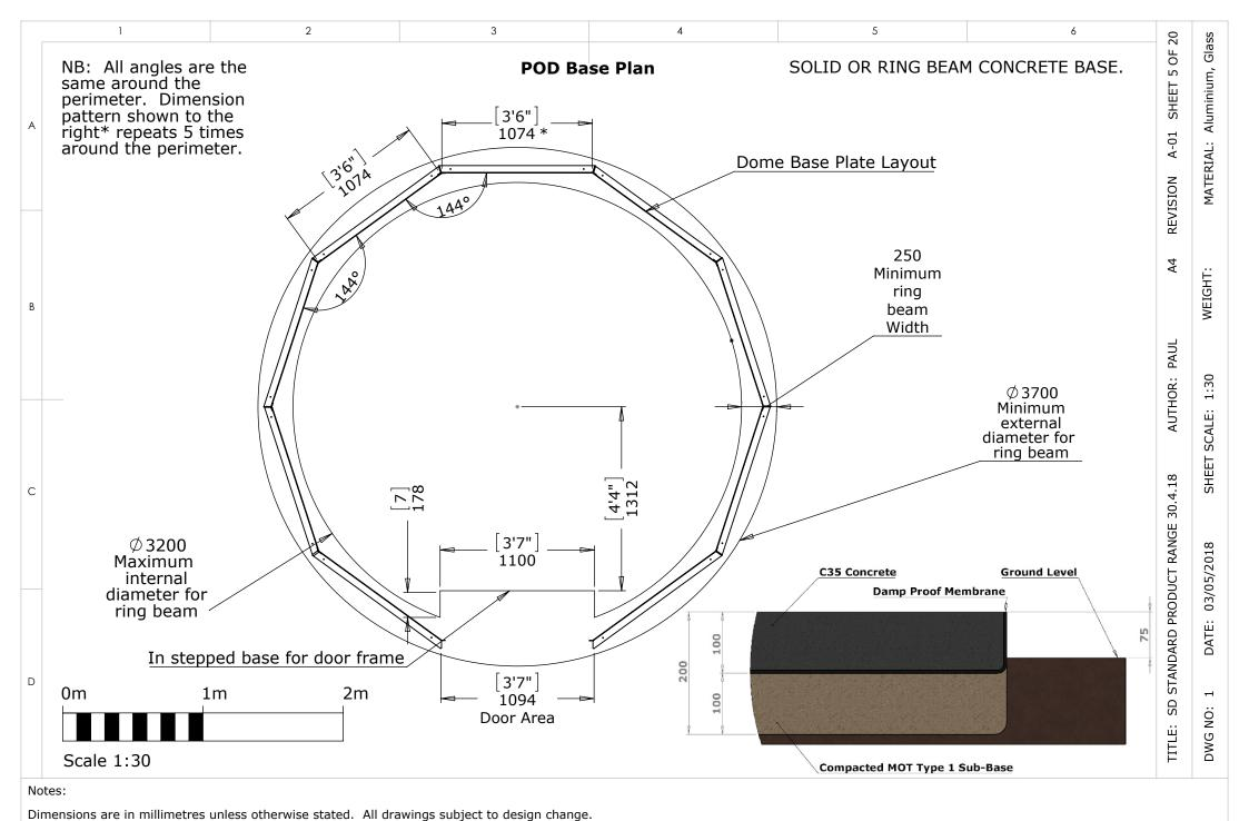
Additional Info: Foundation cross section is recommendation only, based on normal ground conditions.
