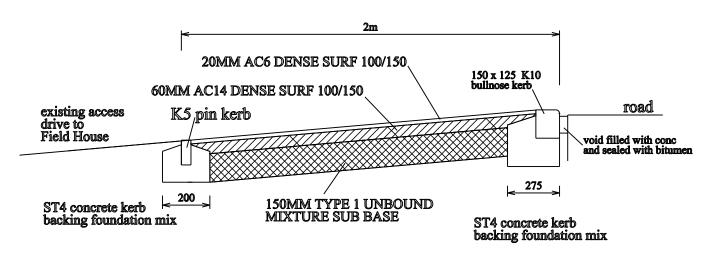
Type A construction section 1:20 scale
