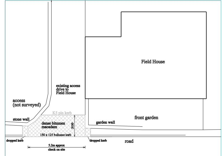
proposed Type A access plan 1:100 scale constructed to northumberland county council highways standards
