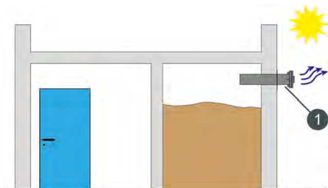
Fig. 12-10: Filling nozzle in open air
