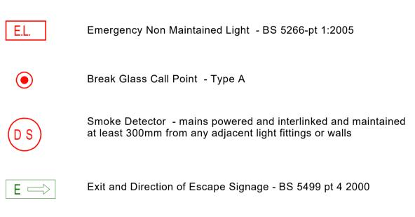
N.B. A combination light box and directional sign may be used as an alternative to seperate fittings
